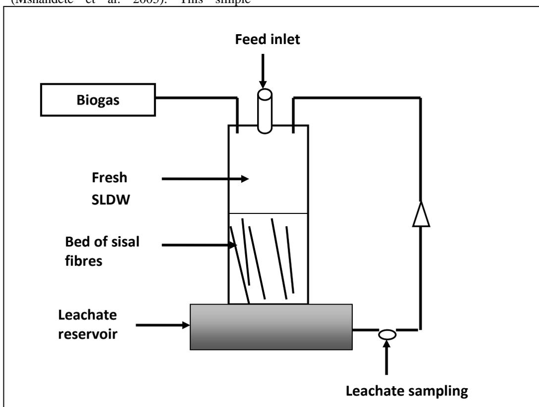
**Figure 1:** Schema of a sisal fibre fixed bed anaerobic digester. SLDW = Sisal leaf decortiations waste
