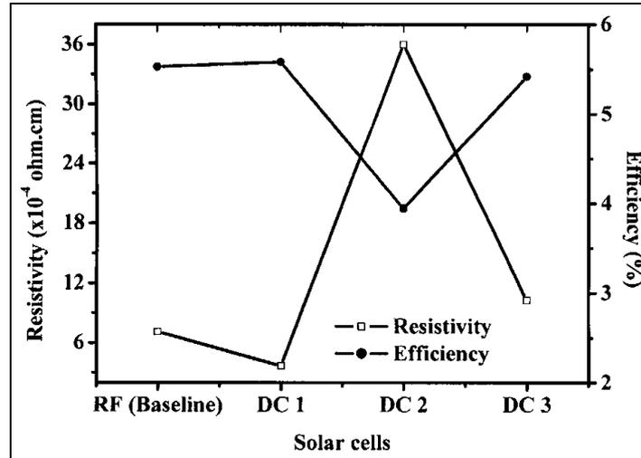
**Figure 5 (a)** The variation of CIGS solar cell efficiencies with their respective ZnO:Al/ZnO double layer resistivities.
