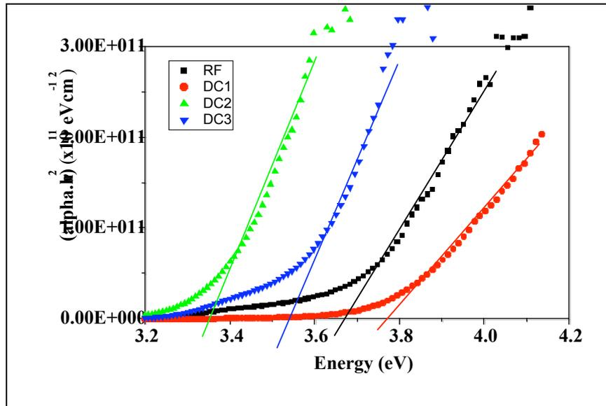
**Figure 4;** The plot of  $(\alpha h\nu)^2$  with energy  $h\nu$  for the determination of optical bandgaps of ZnO:Al/ZnO double layers for RF, DC 1, DC2 and DC3 CIGS solar cells.
