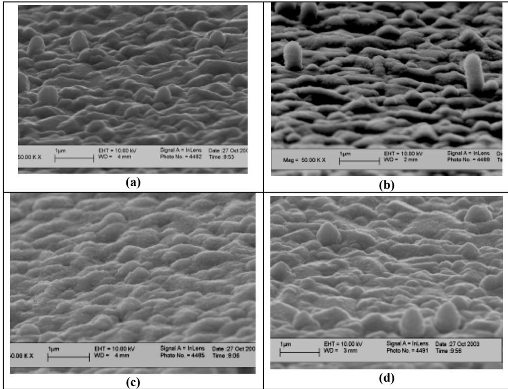
**Figure 1:** SEM plain view images for ZnO:Al/ZnO double layers used to fabricate (a) Baseline (RF) solar cell (b) DC1 solar cell (c) DC2 solar cell and (d) DC3 CIGS solar cell.
