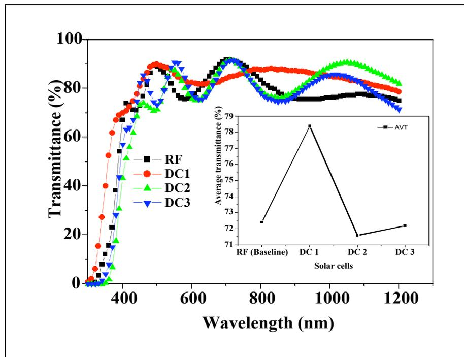
**Figure 3** The transmittance of ZnO:Al/ZnO double layers for RF, DC 1, DC 2 and DC 3 CIGS solar cells
