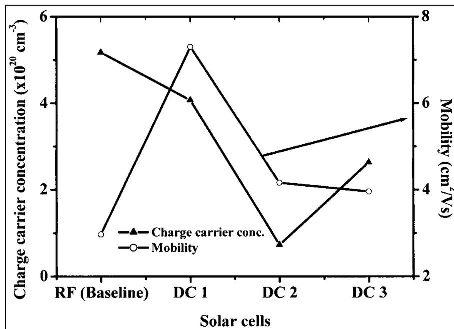
**Figure 6** The variation of ZnO:Al/ZnO charge carrier concentration and mobility with the solar cell efficiency.
